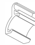
to hold cover plate, installed on either side of the box
